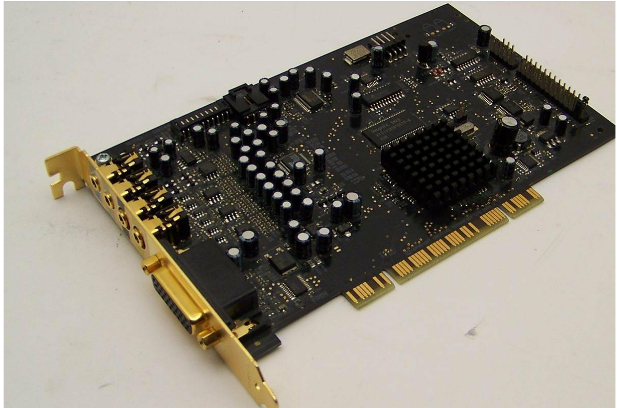
Image 1: The Creative SB0460 sound card, showing its various ports and connectors for audio input and output.
