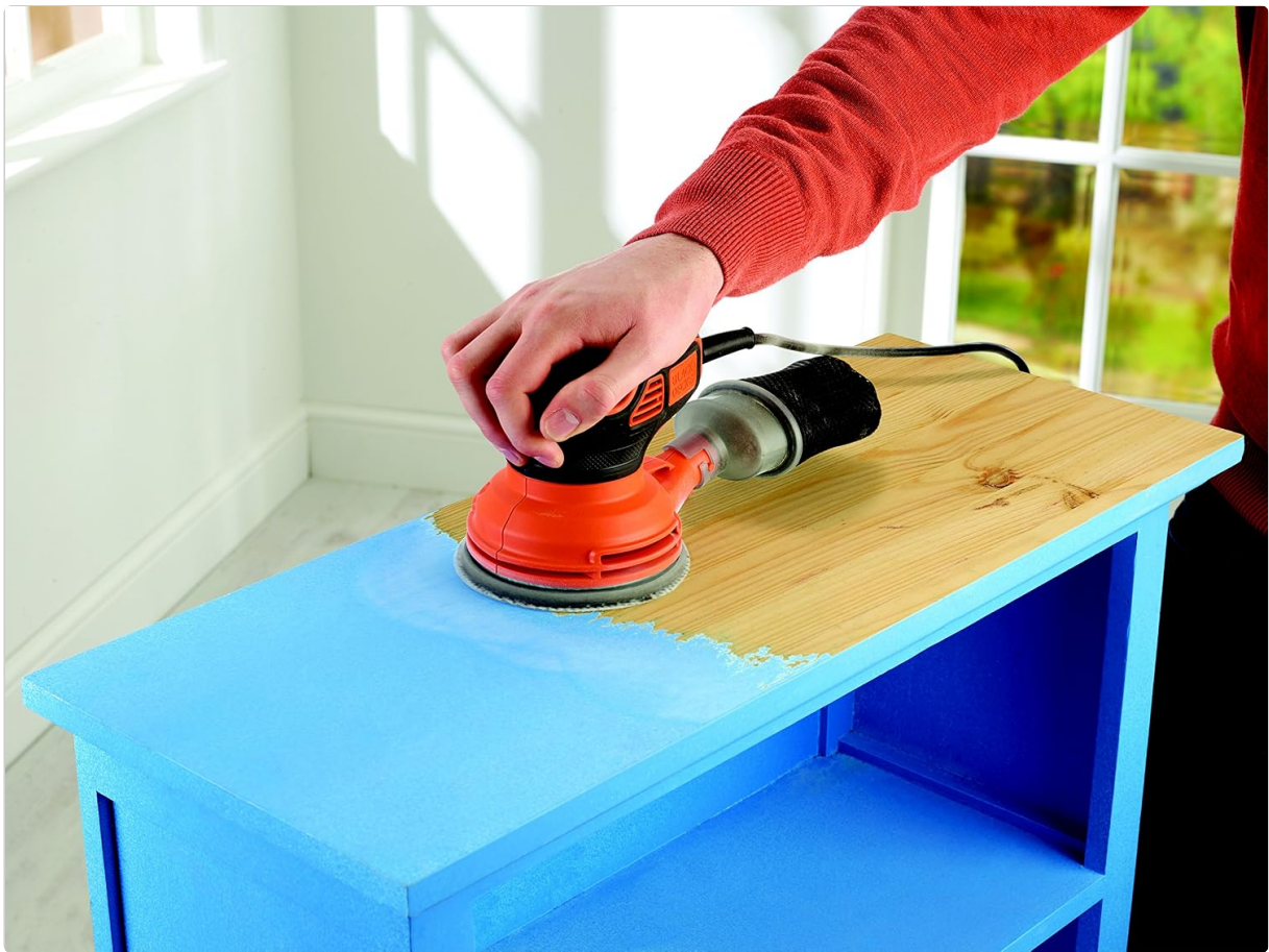
Figure 2: Demonstrating the use of the orbital sander on a painted wooden surface, showing proper hand placement and sanding motion.
