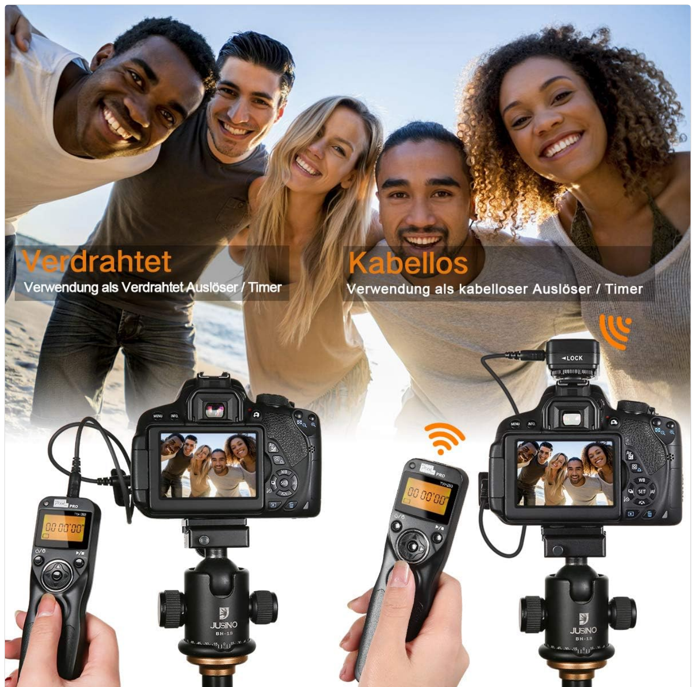
Figure 3.2: Wired and Wireless connection methods. The remote can be used directly wired to the camera or wirelessly via the receiver unit.
