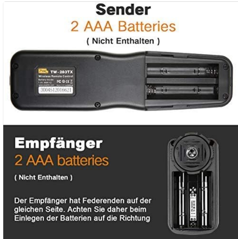
Figure 3.1: Battery compartments for transmitter and receiver. Both units require 2 AAA batteries. Ensure correct polarity during installation.
