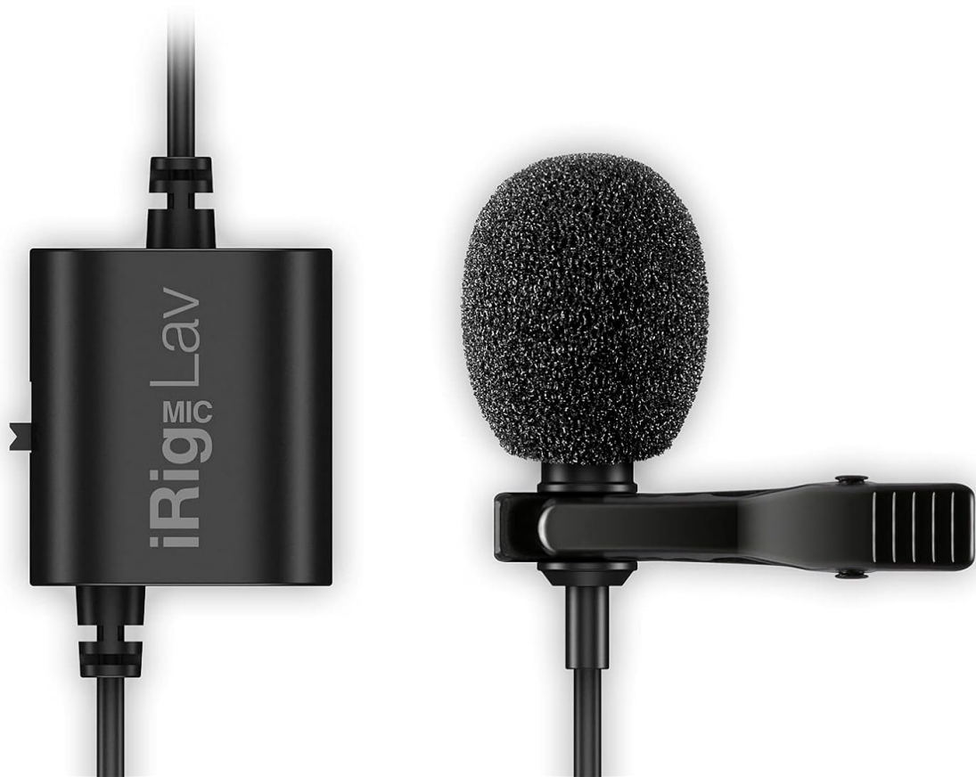
Image 3.1: Detail of the iRig Mic Lav's omnidirectional condenser microphone and clip.
