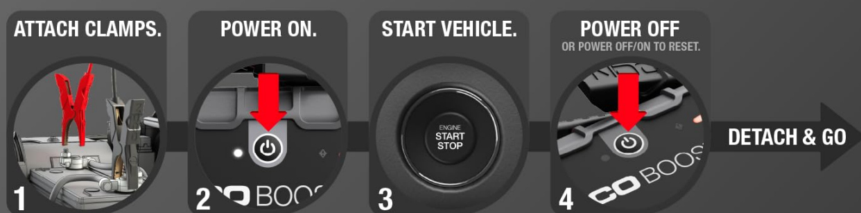
Image: A visual guide demonstrating the four easy steps to use the NOCO Boost GB70: Attach clamps, power on, start vehicle, and detach.
