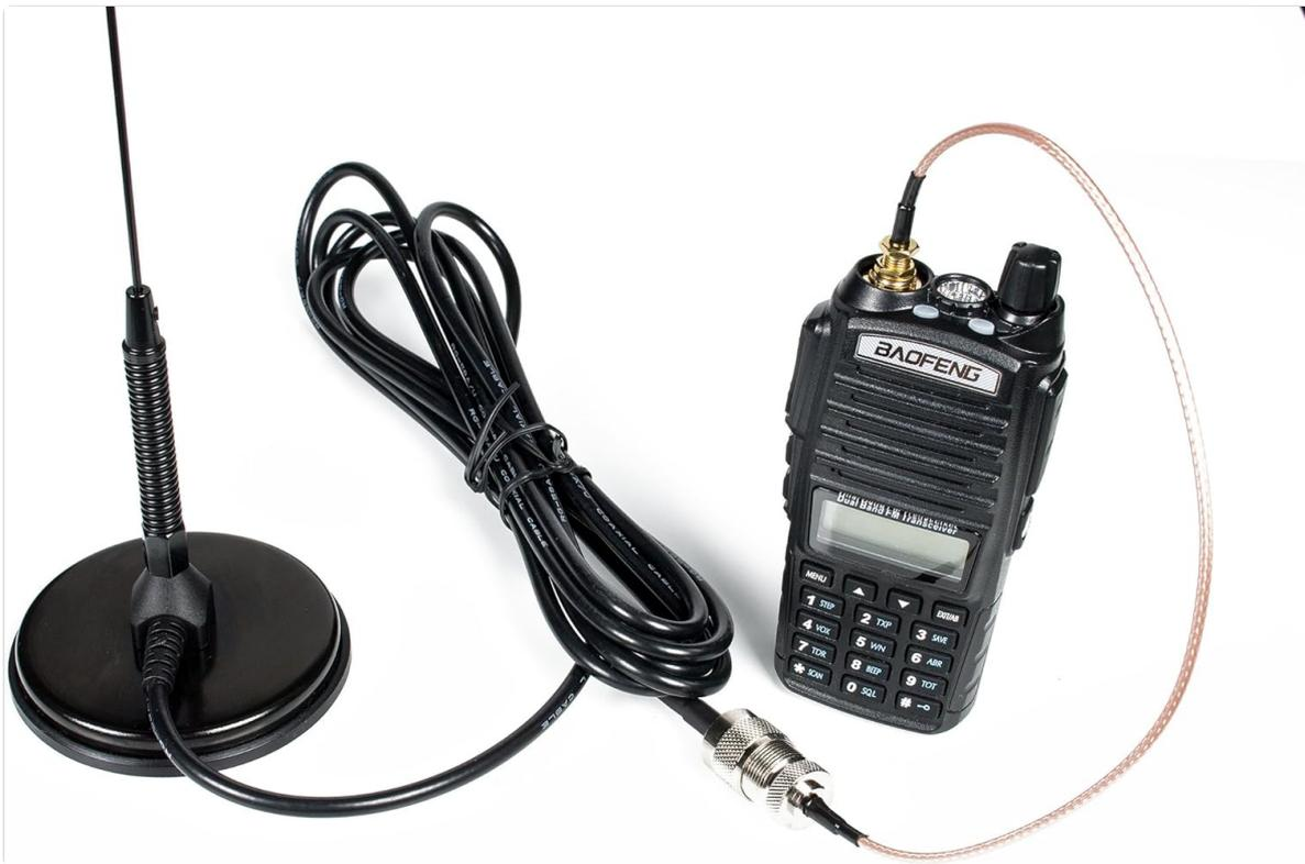
Figure 3: Antenna connected to a handheld radio using the SMA adapter.
