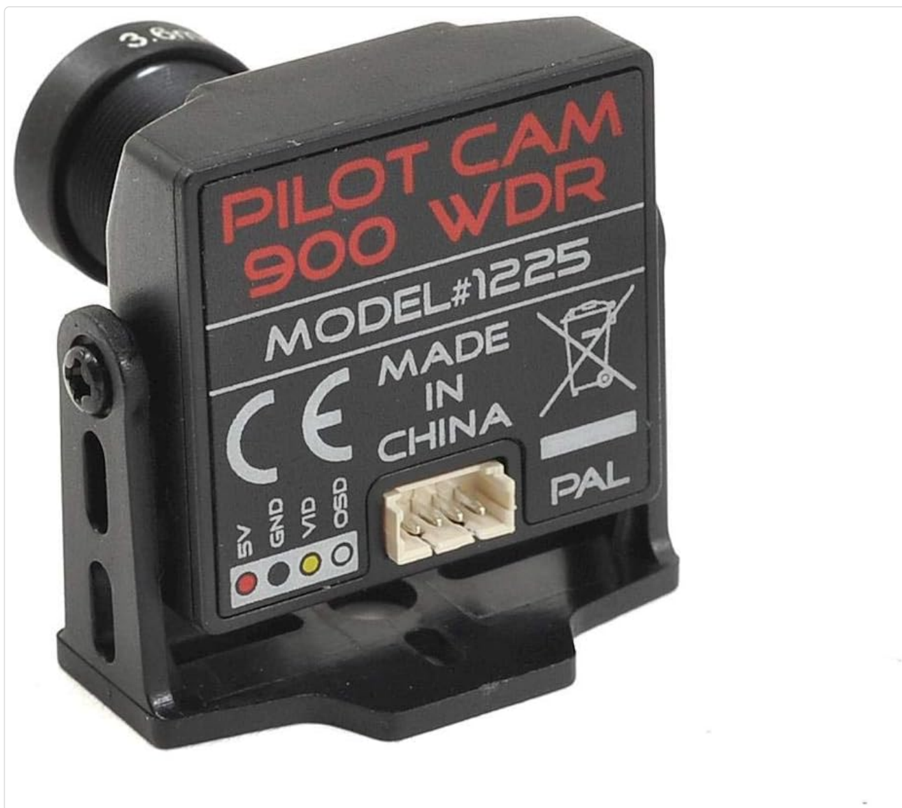
Figure 4.1: Front view of the camera with connection ports labeled.
