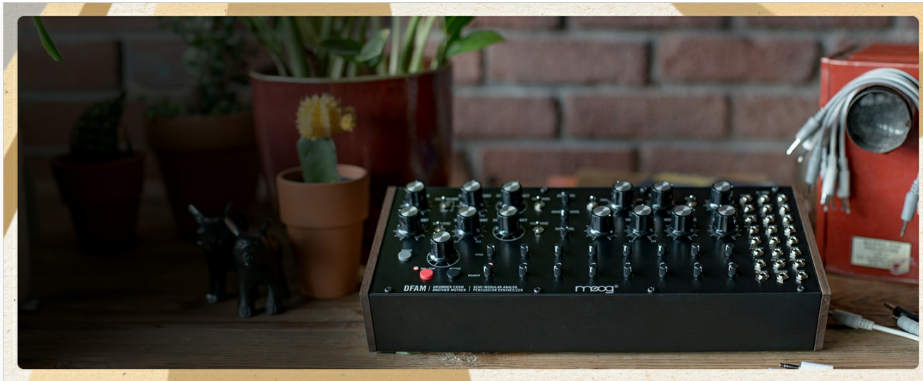
Image 3.4: The 8-step sequencer section of the DFAM, showing Pitch and Velocity controls for each step.
