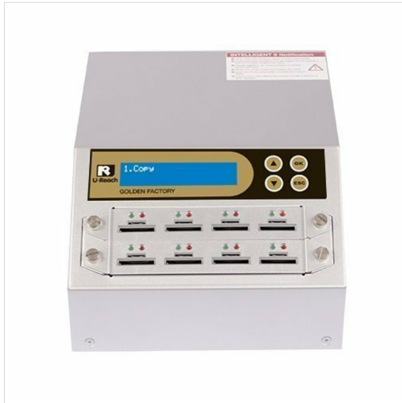
Figure 1: Front view of the U-Reach SD908G Duplicator, showing the multiple SD/mSD card slots and control panel.
