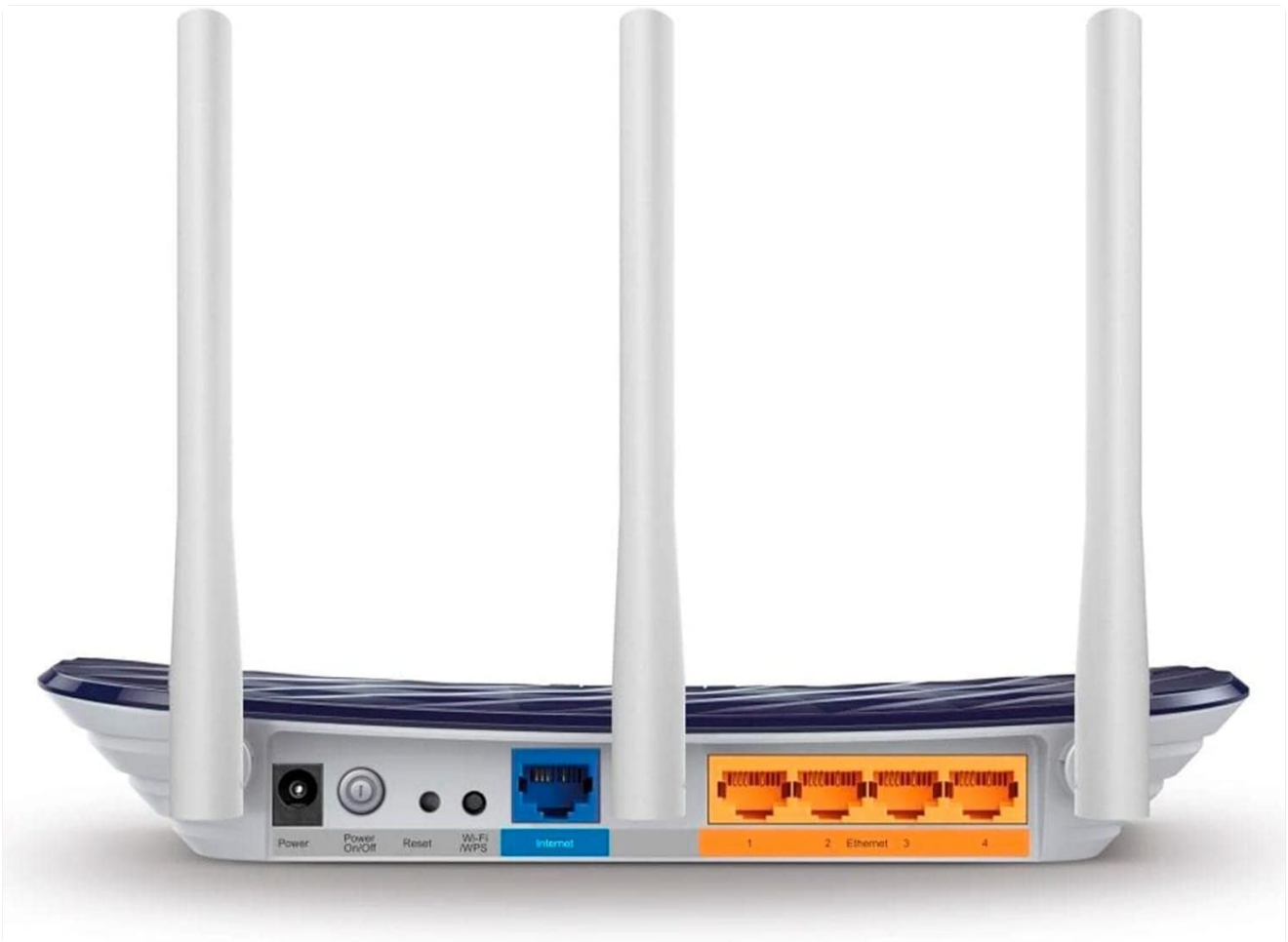
Figure 3.1: Rear panel of the Archer C20, illustrating the power input, power on/off button, Wi-Fi/WPS button, Reset button, blue Internet port, and four yellow Ethernet LAN ports.
