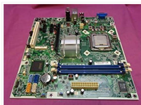
Figure 1: HP 582679-001 Desktop ETON Motherboard. This image displays the overall layout of the motherboard, including the CPU socket, RAM slots, expansion slots, and various connectors.
