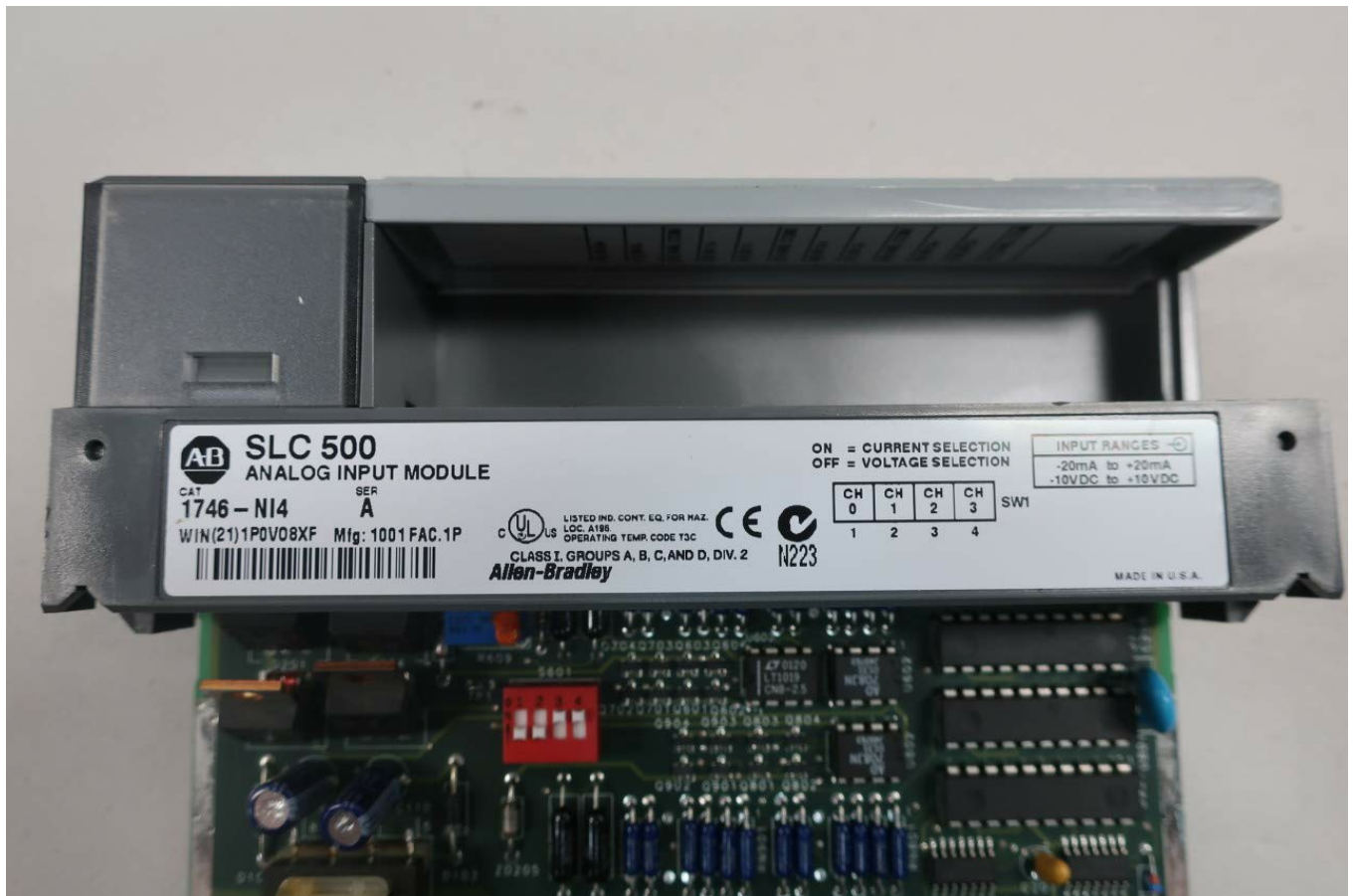
Figure 3: A detailed view of the product label on the 1746-NI4 module. This label specifies the catalog number (CAT: 1746-NI4), series (SER A), and provides a table for input range selection via DIP switches (SW1), indicating options for current (-20mA to +20mA) and voltage (-10VDC to +10VDC) inputs.
