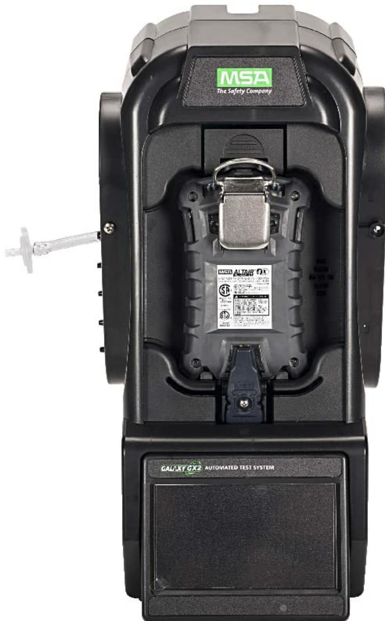
The image shows an MSA ALTAIR 4/4X multi-gas detector securely placed within the MSA Galaxy GX2 Automated Test System, ready for calibration or functional testing.
