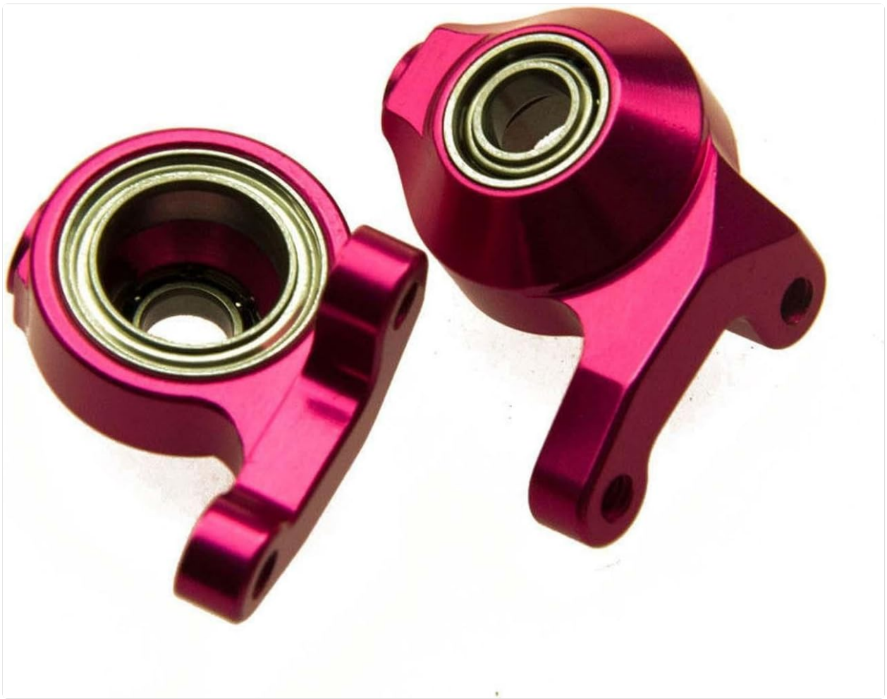
Image 5.1: Angled view of the steering hubs, highlighting mounting points.
