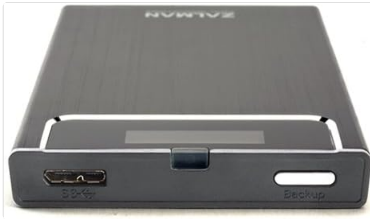
Image: Top view of the Zalman ZM-VE350 HDD Enclosure, highlighting the USB 3.0 port (S3-4) and the jog-switch button on the side, along with a "Backup" button.
