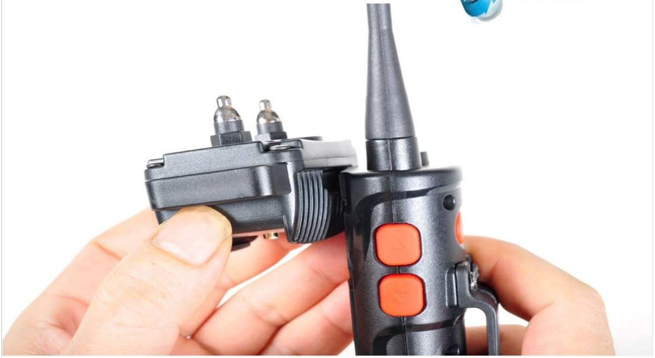
Image 3.3: Remote and Receiver Collar connection points.
