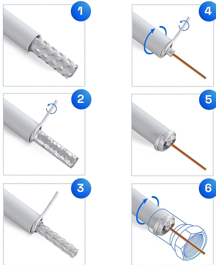
Image 3.1: Visual guide for F-connector installation.
