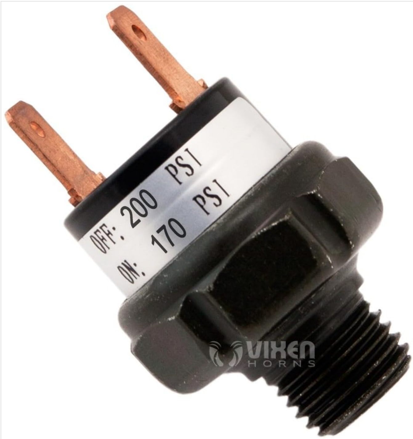
The pressure switch, designed to activate the compressor at 170 PSI and deactivate it at 200 PSI.
