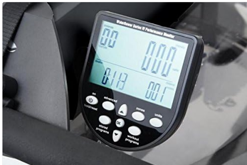
Figure 4: Close-up of the WaterRower S4 Performance Monitor display. The screen shows various workout metrics such as stroke rate, intensity, time, and distance, with buttons for navigation and program selection.
