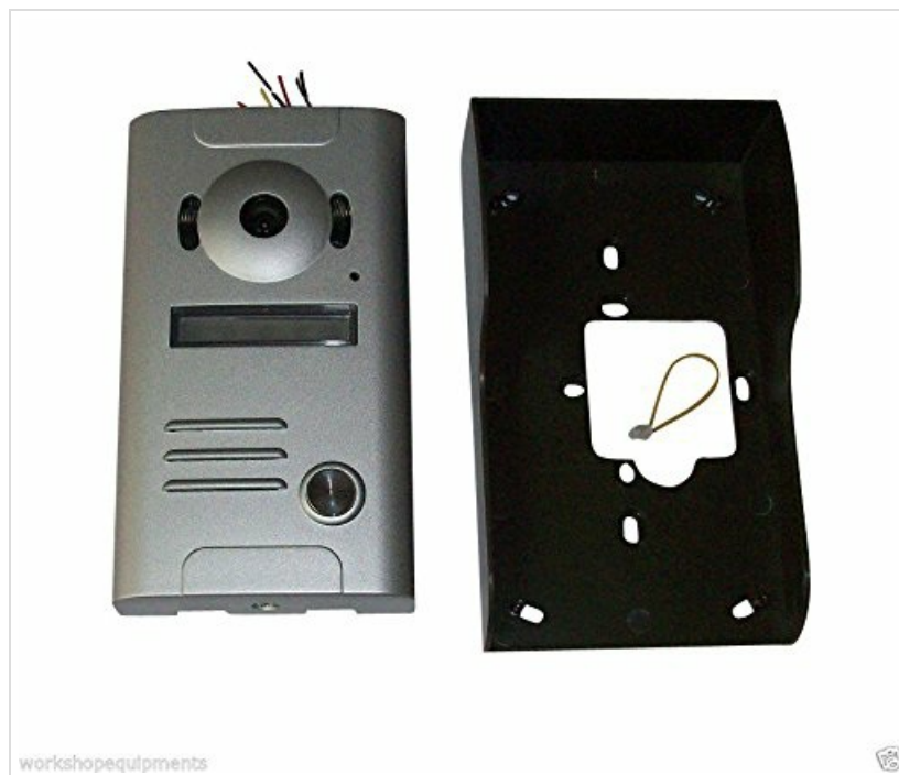
Figure 3.2: Front view of the ZHUDELE ZDL-M outdoor unit, featuring the camera, speaker, microphone, and call button.
