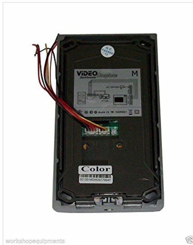
Figure 3.3: Rear view of the ZHUDELE ZDL-M outdoor unit, displaying the wiring connections and internal components.
