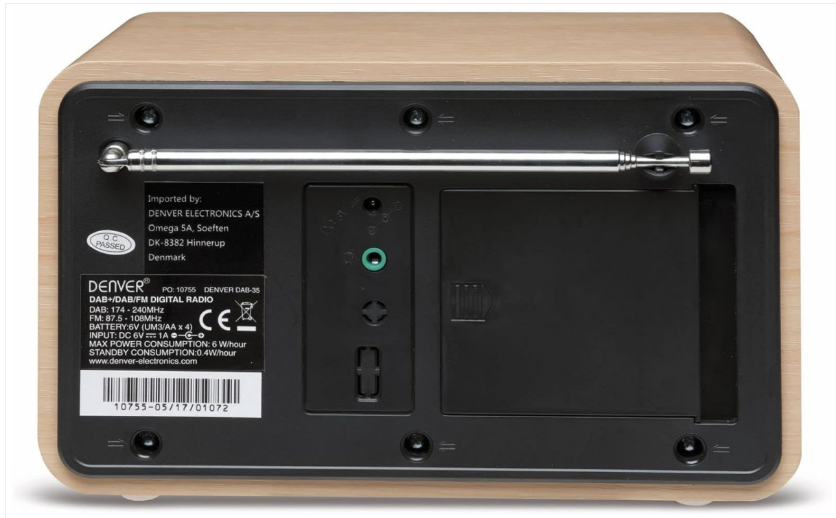
Figure 3.3: Rear view of the Denver DAB-35 radio, showing the telescopic antenna, power input, and headphone jack.
