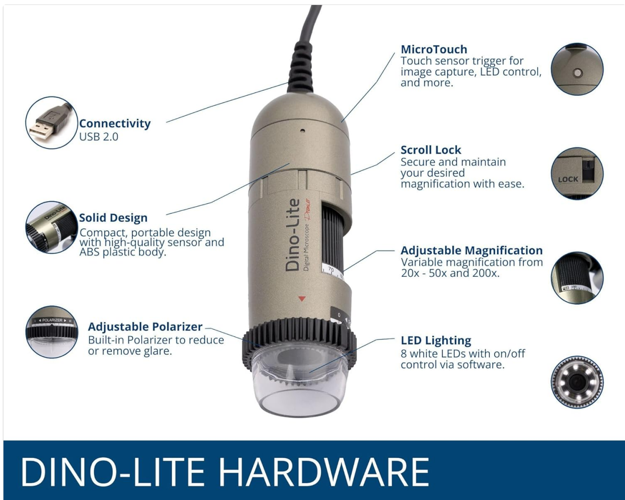
Image 1.3: Detailed illustration of the Dino-Lite AM4113ZT hardware, highlighting its various components and their functions.
