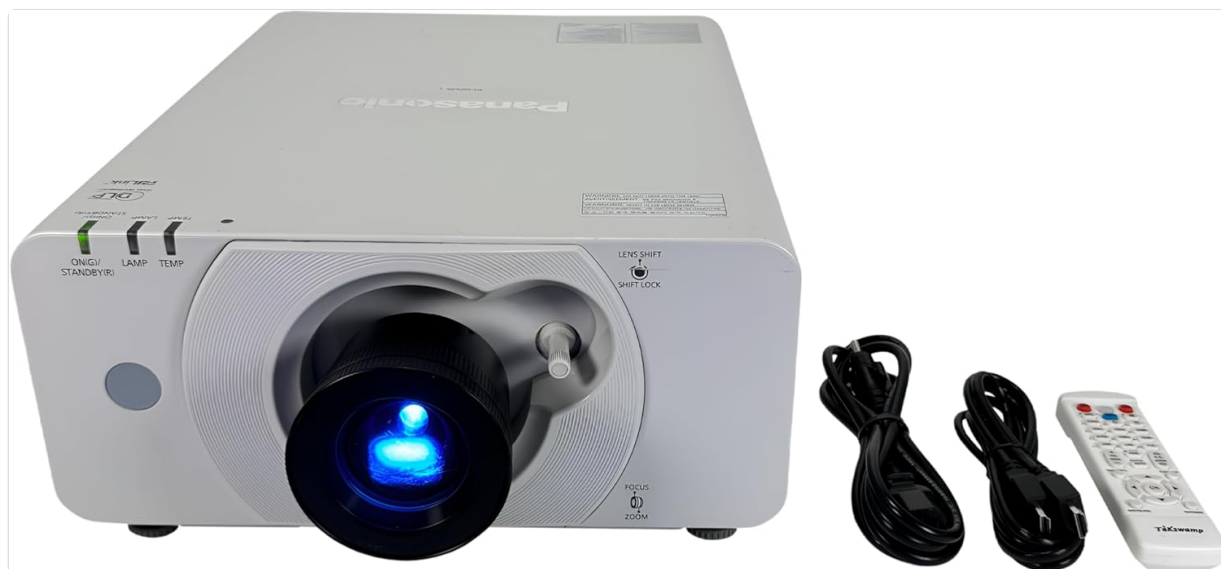
Figure 4.1: Panasonic PT-DZ570U DLP Projector, showing the front lens, top panel indicators, and included accessories.
