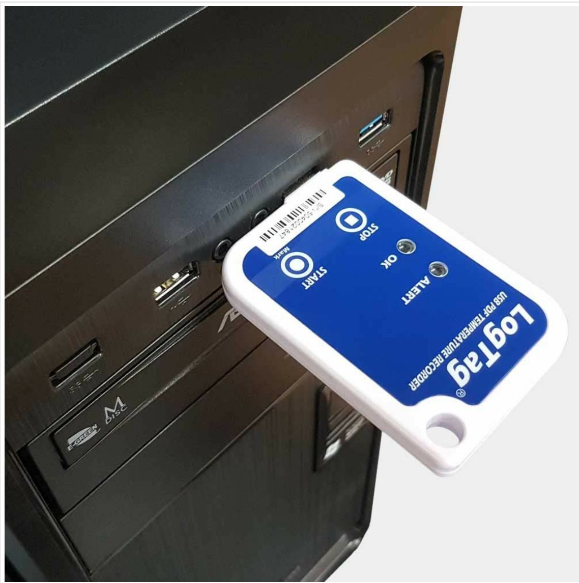
Figure 3: The LogTag UTRIX-16 data logger connected to a computer's USB port. This illustrates the direct connection method for data download and configuration, eliminating the need for a separate interface cradle.
