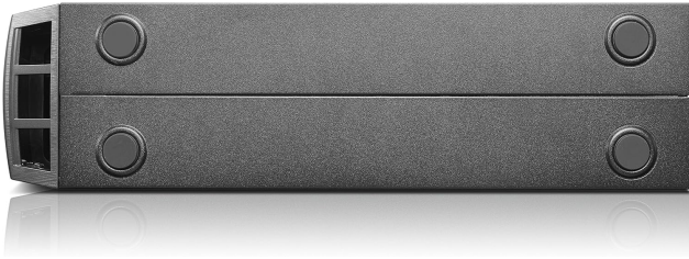
Figure 2.6: Bottom view of the desktop, revealing the rubber feet for stability.
