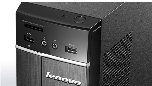
Figure 2.8: Close-up of the power button located on the top right of the front panel.
