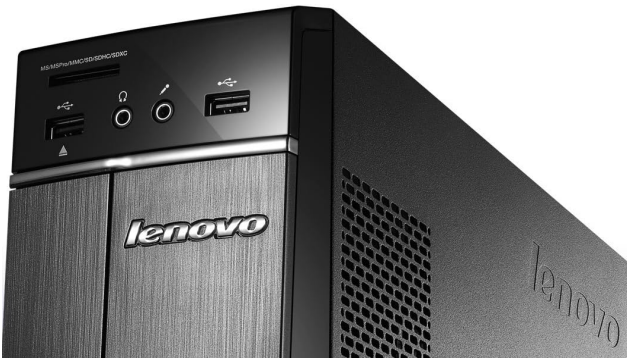
Figure 2.7: Close-up of the front panel, showing USB ports, headphone and microphone jacks, and a multi-card reader.
