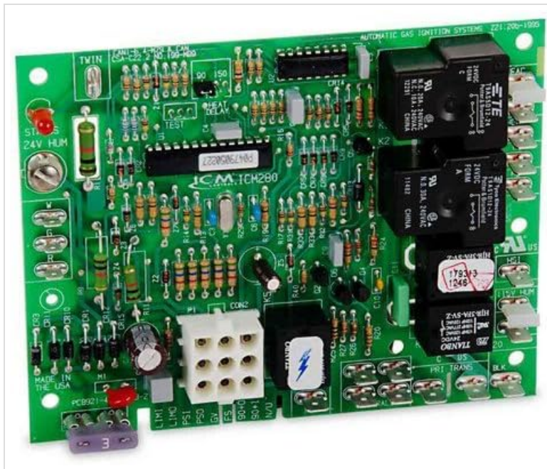
Figure 1: Overview of the Goodman Furnace Control Circuit Board. This image displays the green circuit board populated with various electronic components, including relays, resistors, capacitors, and integrated circuits, along with multiple connectors for wiring harnesses. Key labels such as "TEST" and "24V HUM" are visible, indicating diagnostic and functional points.
