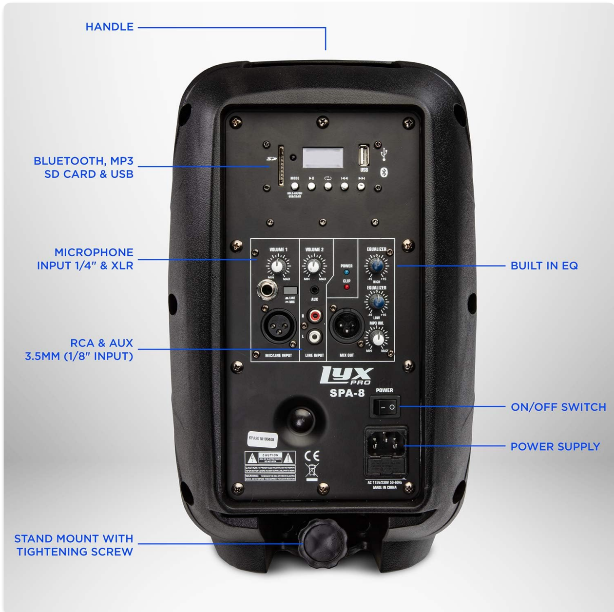
Figure 5: Rear panel showing various inputs, outputs, and controls.
