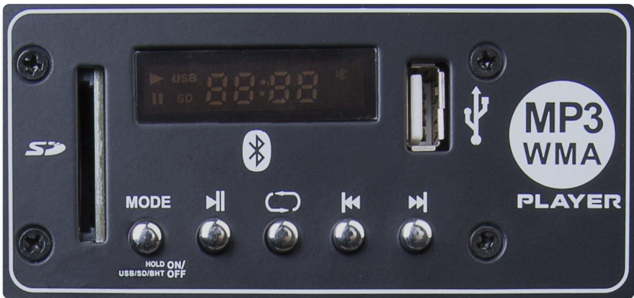
Figure 8: MP3 player section with SD card slot, USB port, and playback controls.
