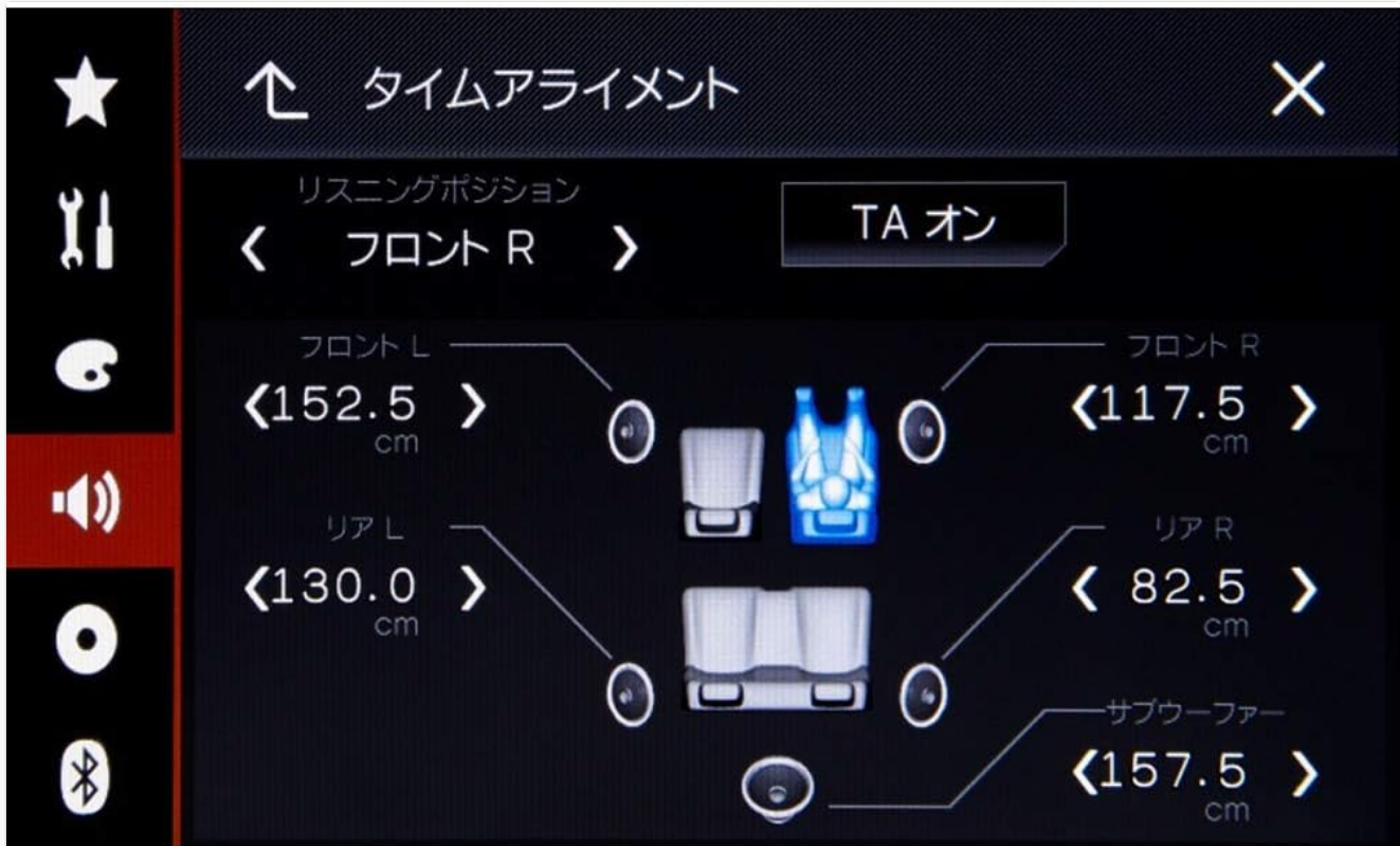
Figure 3: Time Alignment adjustment screen, showing speaker distance settings.
