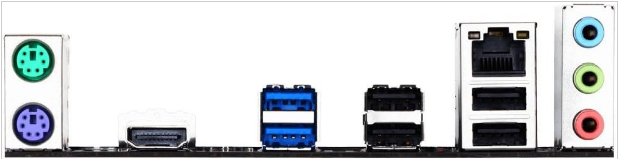
Close-up of the rear input/output (I/O) panel of the GIGABYTE GA-H110M-A motherboard, featuring PS/2 ports, HDMI, USB 3.0, USB 2.0, Ethernet, and audio jacks.
