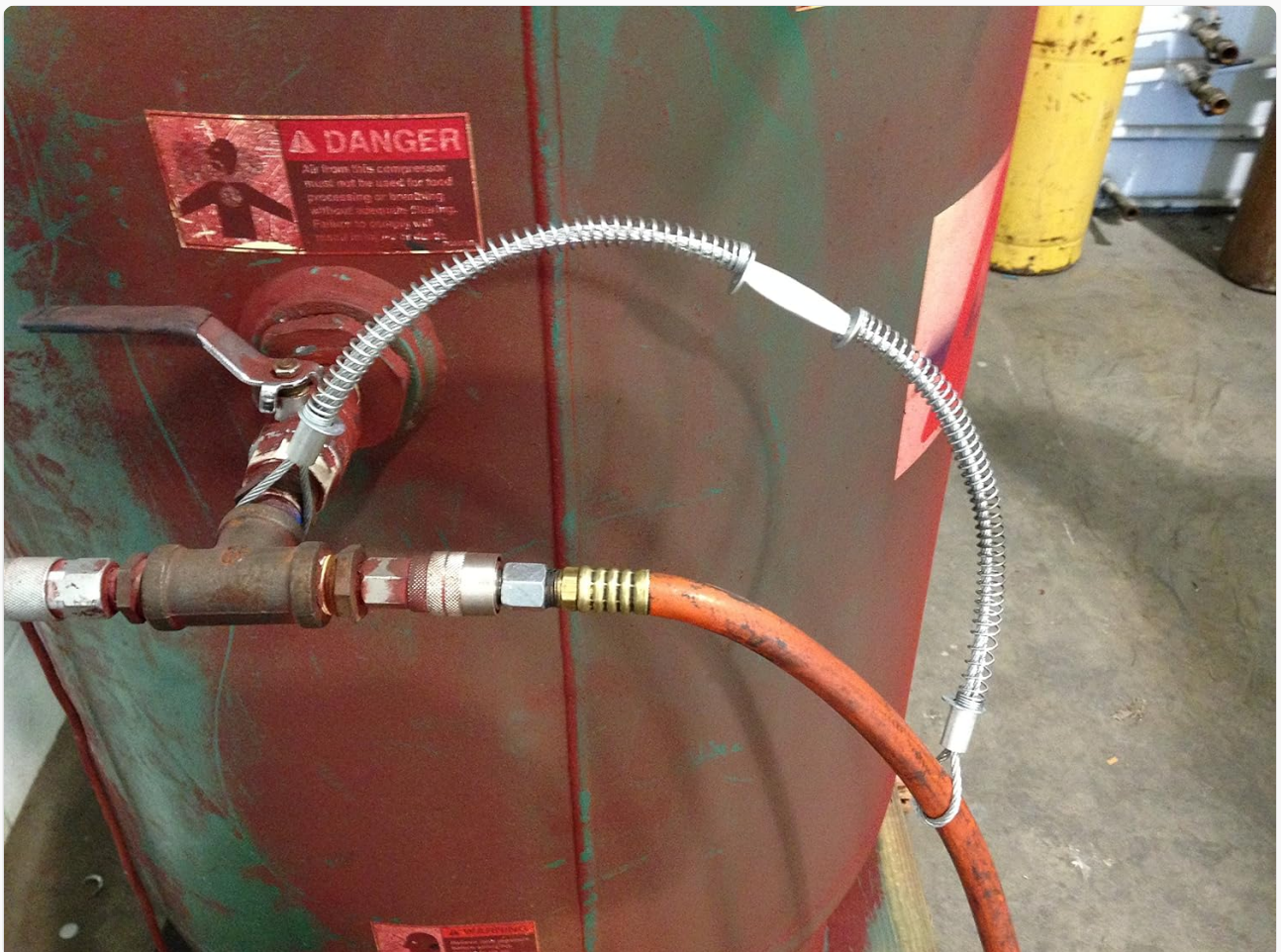
Image: A WC-4 Whip Check properly installed on a hose connection, showing the cable looped around the hose near the
