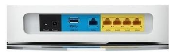
Figure 4.2: Rear panel of the Huawei WS880 router. From left to right, it includes a recessed Reset button, a Power input jack, a blue USB 3.0 port, a blue WAN port, and four yellow Gigabit LAN ports.
