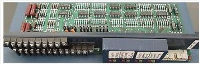
Figure 1: ADT Fire Alarm Circuit Board 4520-330. This image displays the top view of the circuit board, highlighting its integrated circuits, resistors, capacitors, and the terminal blocks for wiring connections.
