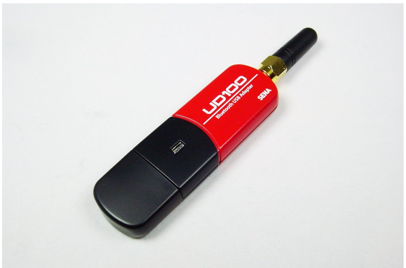
Figure 3.2: Parani-UD100 Adapter with the antenna securely attached, ready for use.
