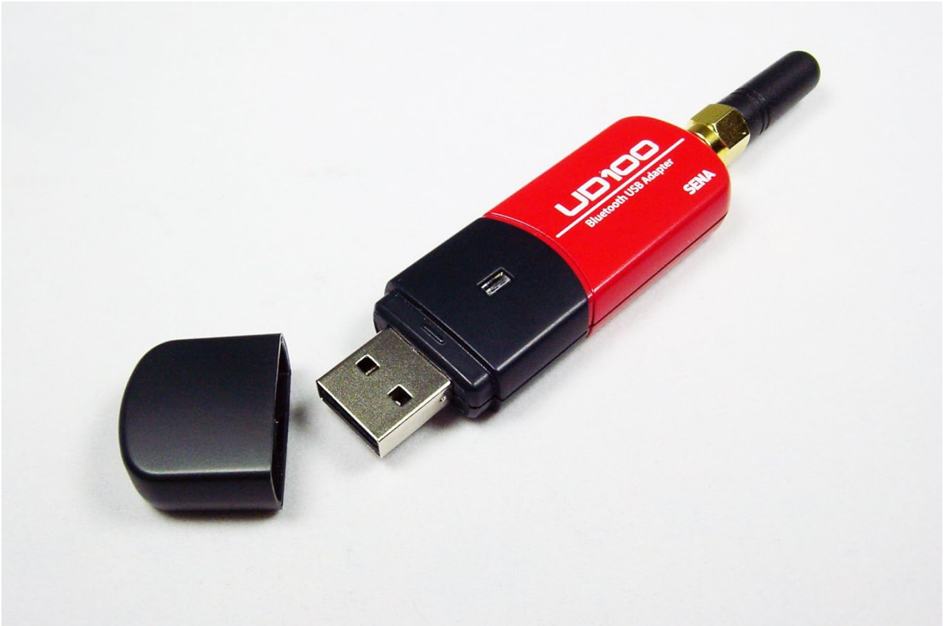
Figure 3.3: Parani-UD100 Adapter with its protective cap removed, revealing the USB connector.
