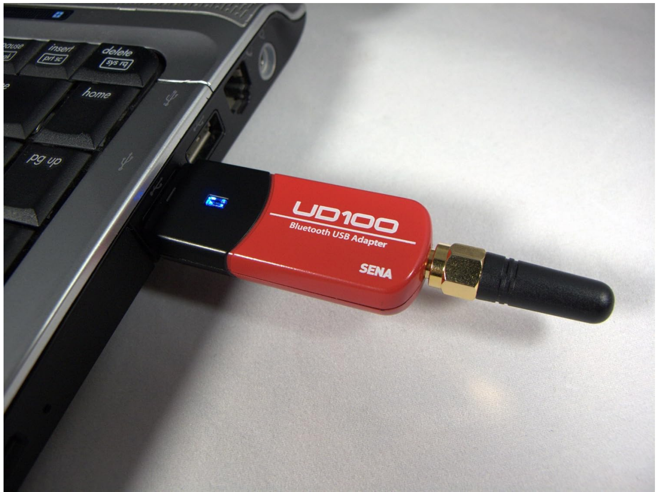
Figure 4.1: Parani-UD100 Adapter correctly inserted into a laptop's USB port, indicated by the blue LED.
