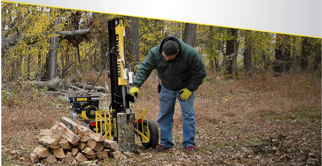
Figure 3: Operating the log splitter in vertical mode to split a log.
