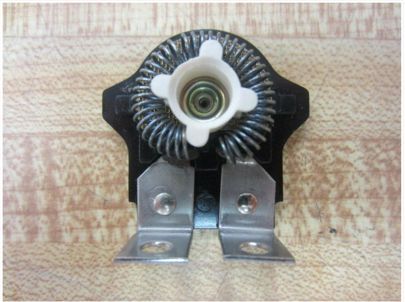
Figure 3.2: Detailed view of the heating element and terminals of the thermal unit.
