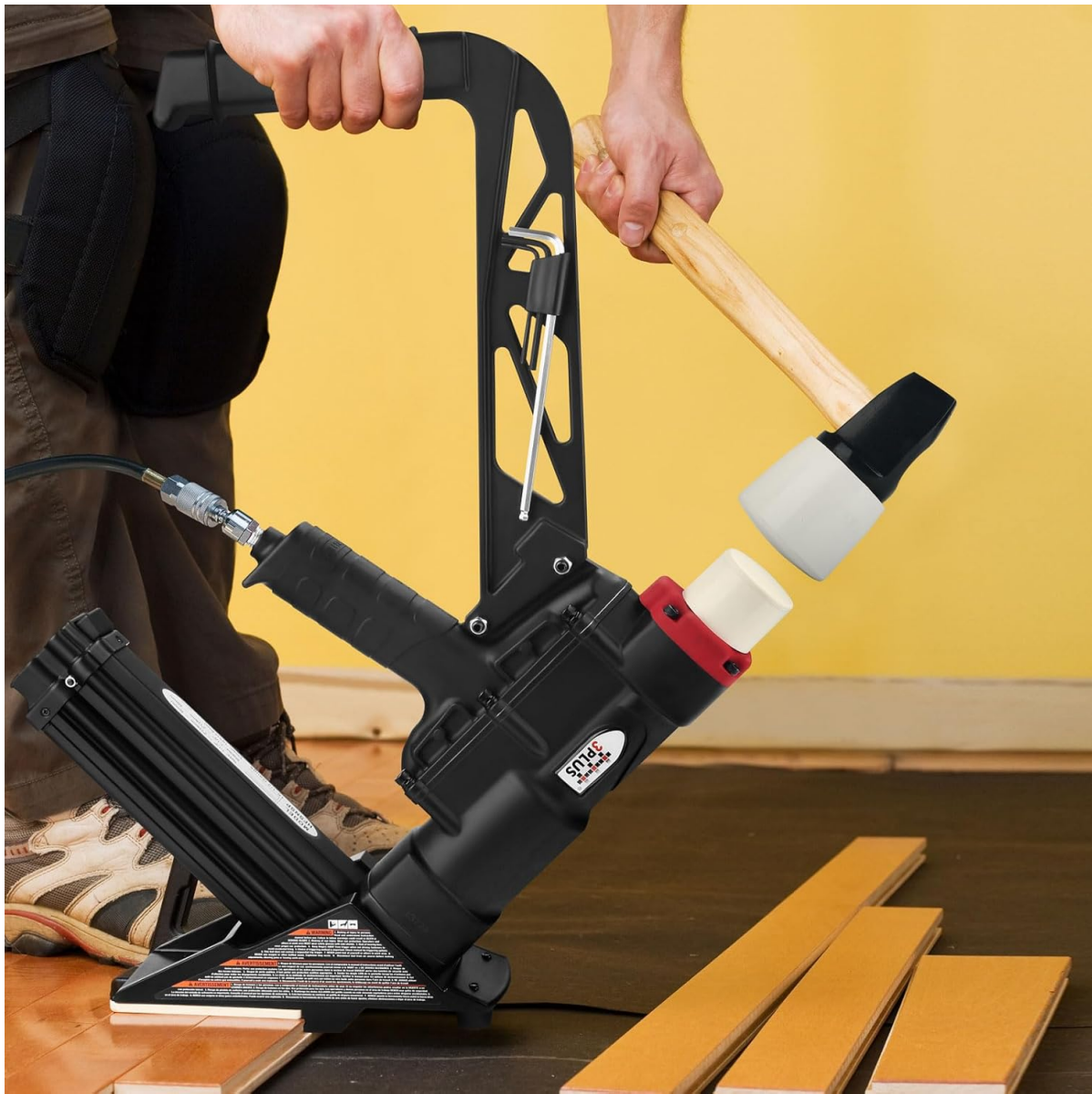
Figure 8: A user striking the tool's cap with the mallet to drive a fastener, illustrating the pneumatic operation.
