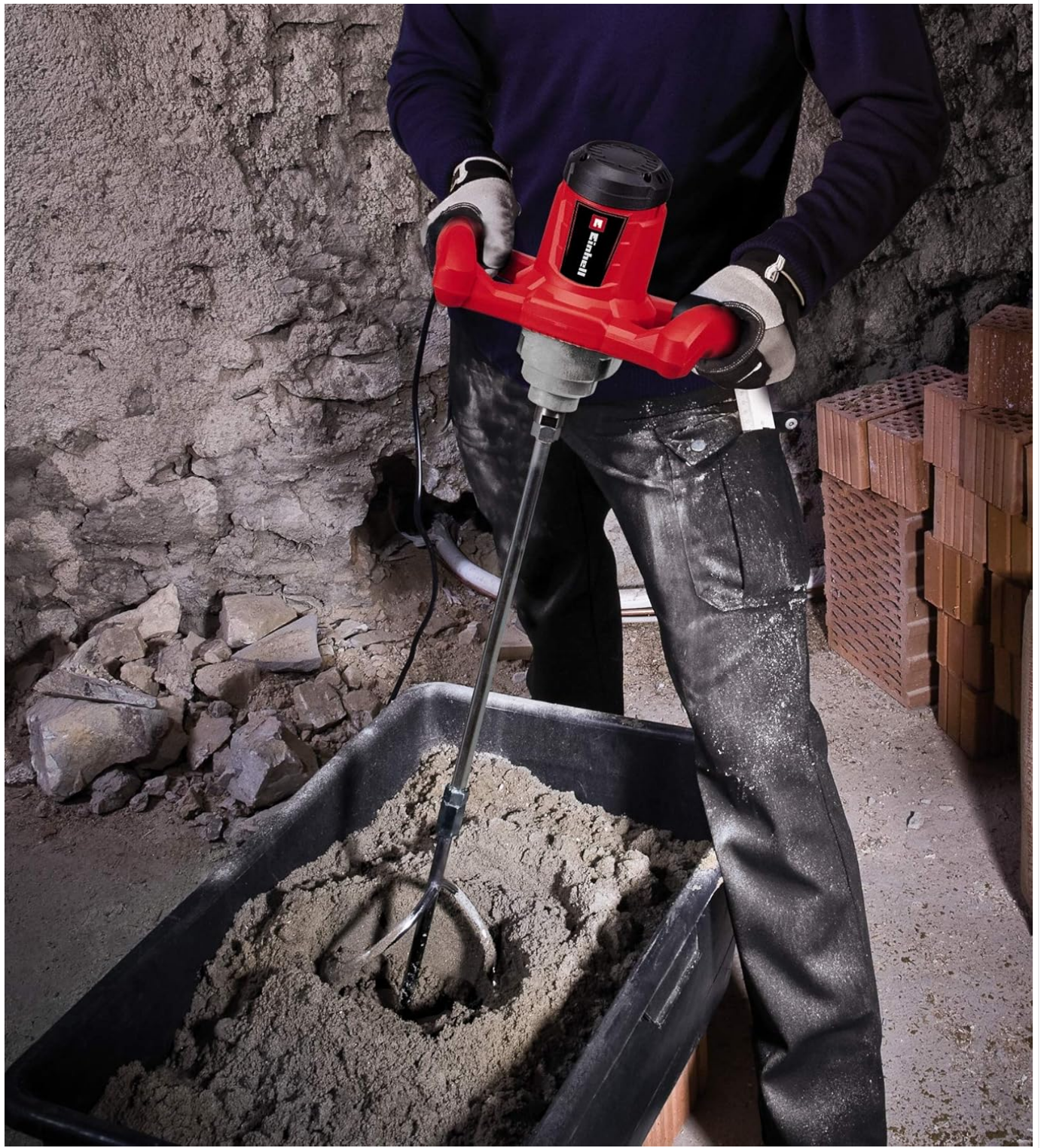
Figure 5: A user demonstrating the proper technique for mixing materials in a tub, holding the mixer firmly with both hands.
