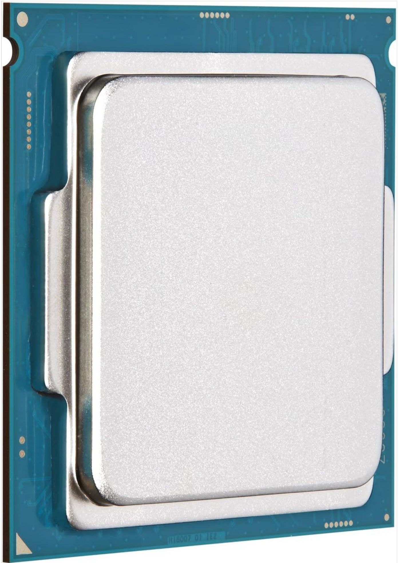
Figure 3.1: Top view of the Intel Core i3-6100 Processor, showing the integrated heat spreader (IHS).
