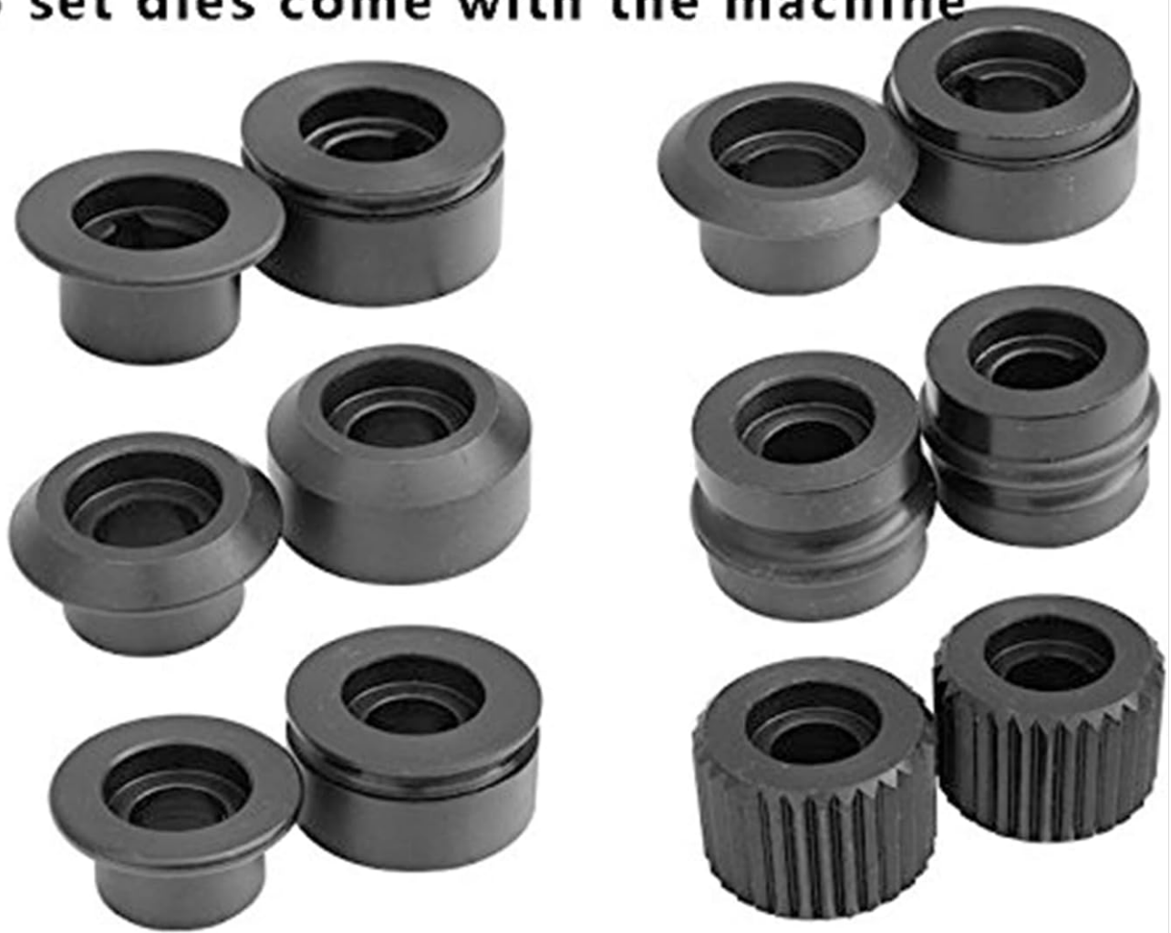
Figure 3.2: The six sets of forming dies included with the RM-08 machine.
