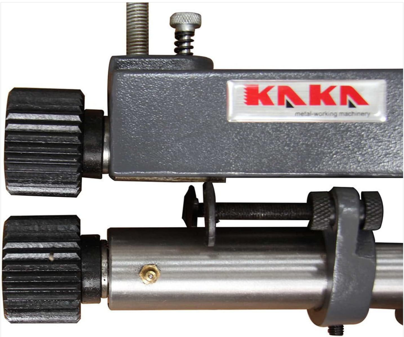
Figure 5.2: The top knob for adjusting forming depth and roll pressure.
