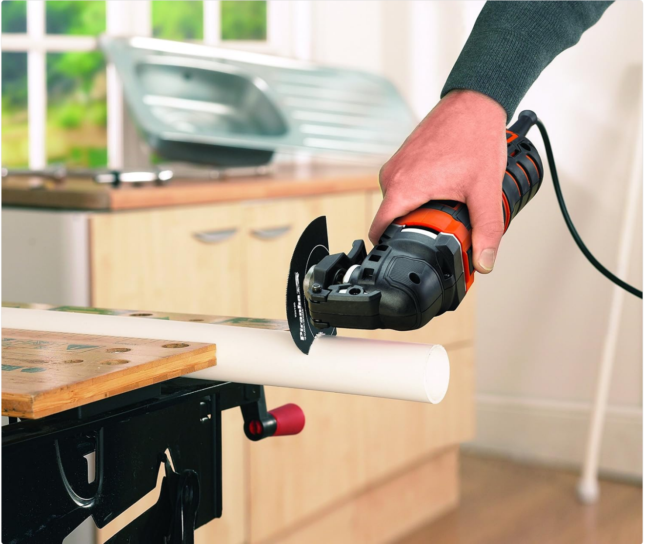
Figure 6.1: The multi-tool being used to precisely cut a PVC pipe, demonstrating its utility for plumbing or similar tasks.
