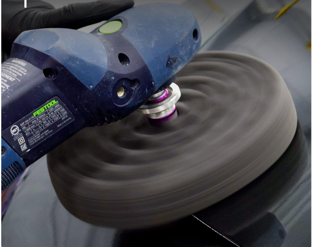
Image 4.2: Close-up view of the polishing process, demonstrating the polish's adherence to the pad and minimal sling.
