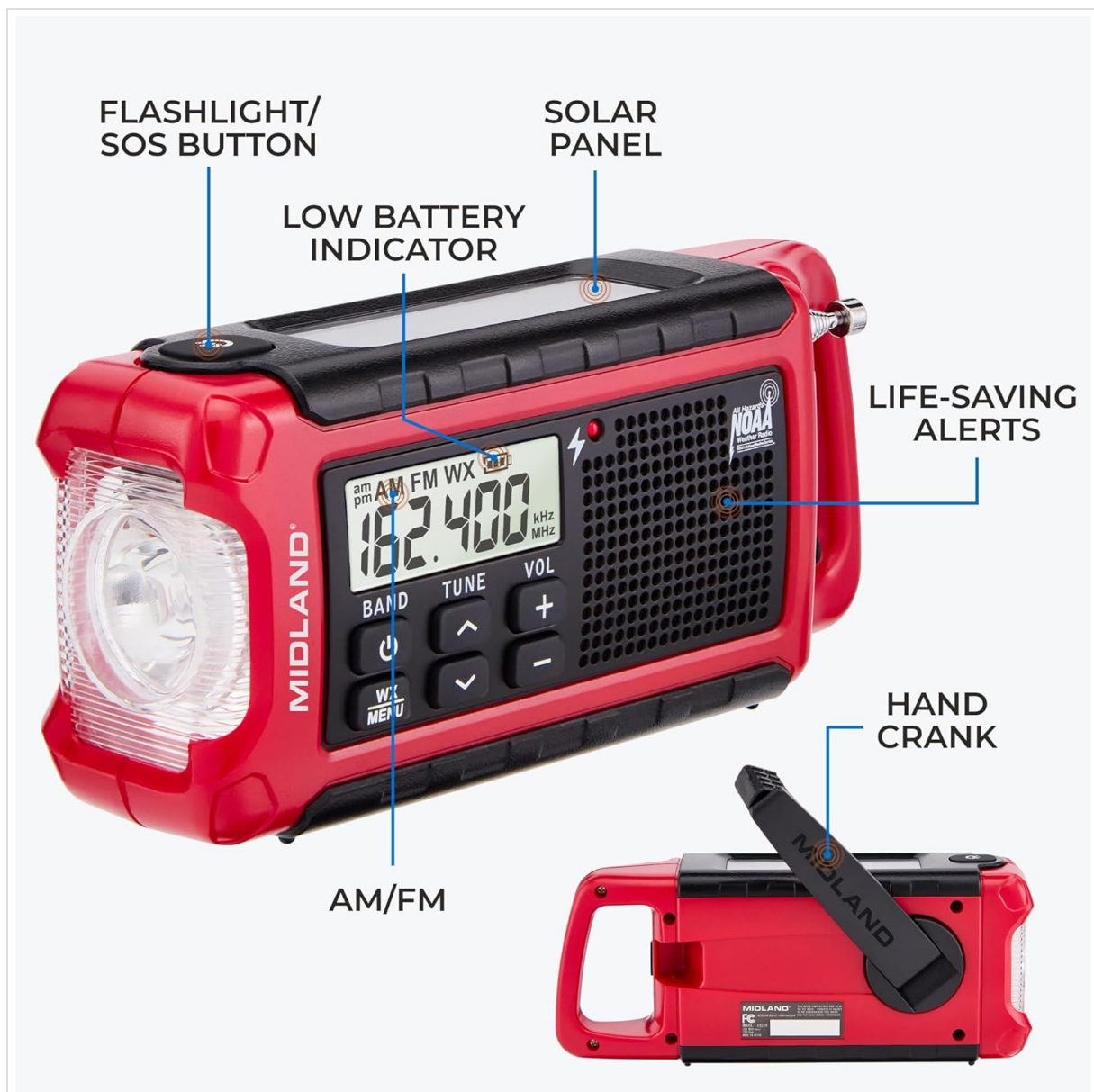
Figure 1: Midland ER210 with key features labeled.
