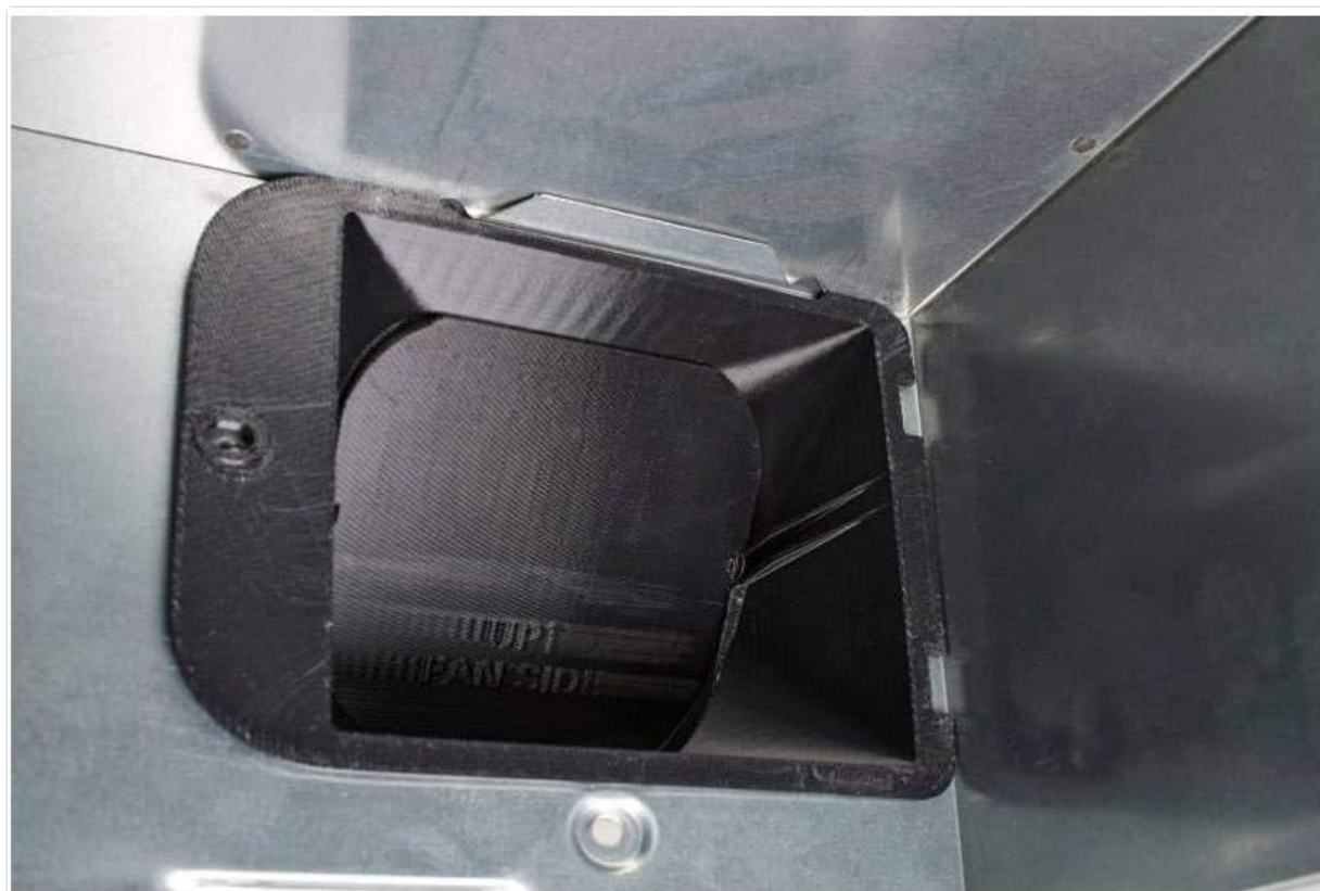
Image: A close-up view of the internal damper mechanism, which should be kept clear of obstructions.
