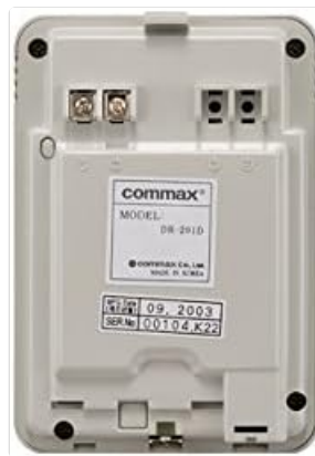
Figure 3.2: Rear view of Commax DR-201D Doorbell Unit showing wiring terminals and model label. This image shows the back of the outdoor unit, indicating its wiring terminals and product identification label.
