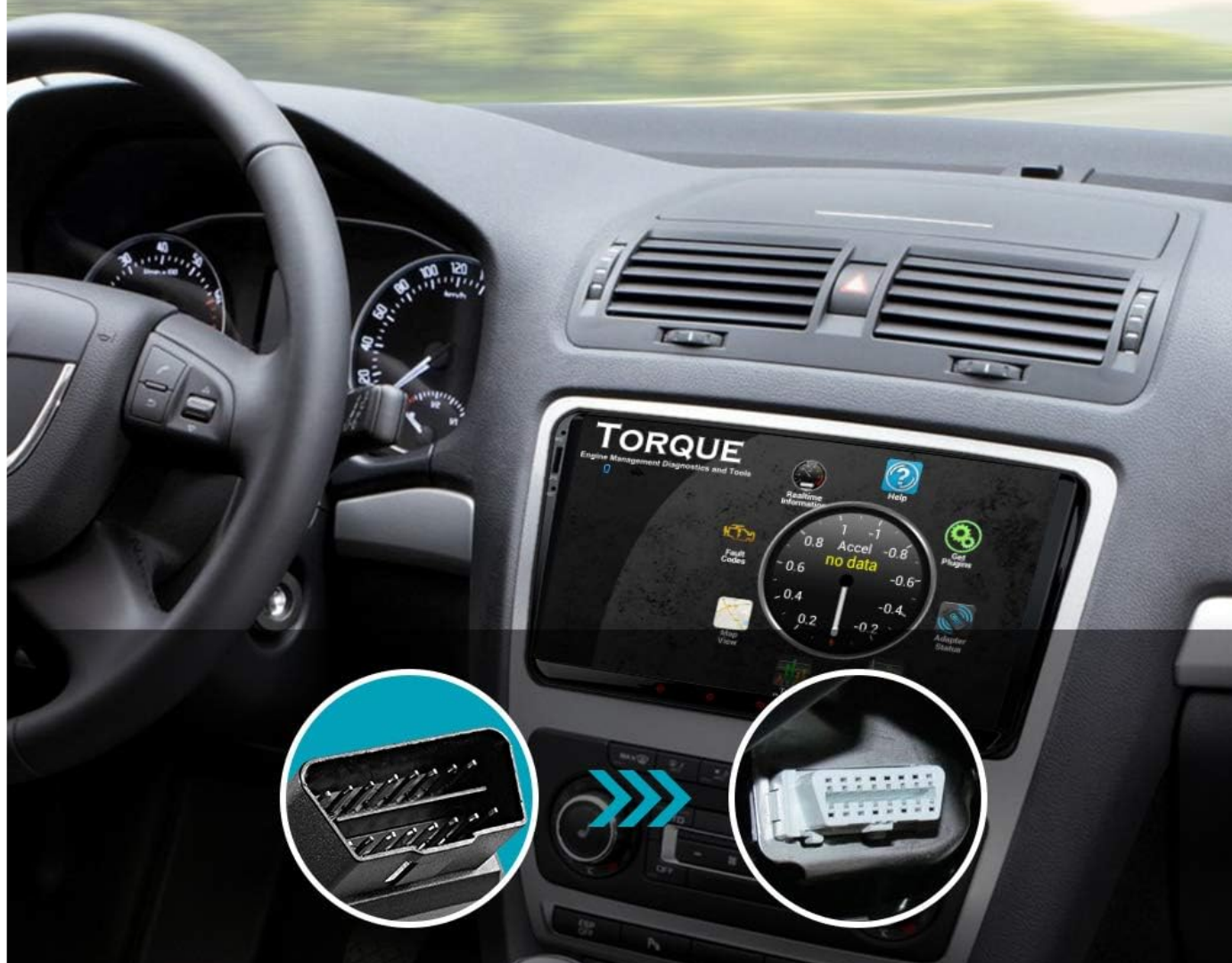
Image: Illustration showing the typical location of a 16-pin OBD2 connection port in a vehicle, usually under the dashboard.
