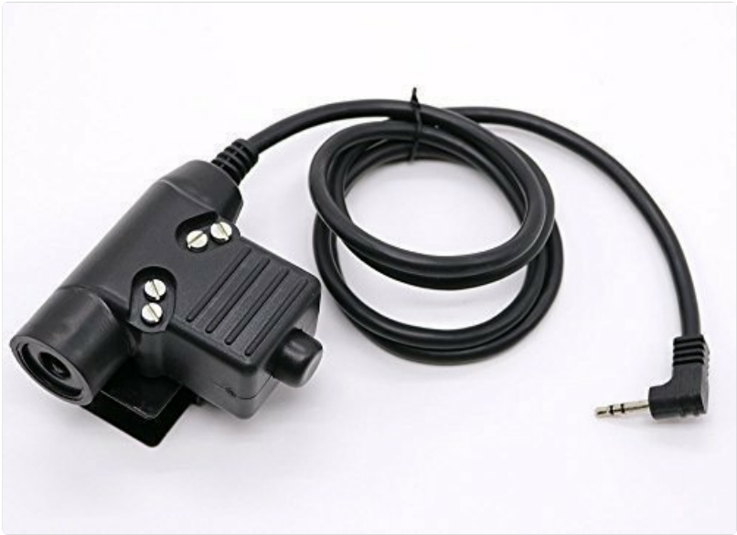
Image: Z-Tactical U94 PTT Military Adapter with 2.5mm Motorola connector. This image shows the overall adapter unit, including the PTT button and the coiled cable leading to the radio connector.
