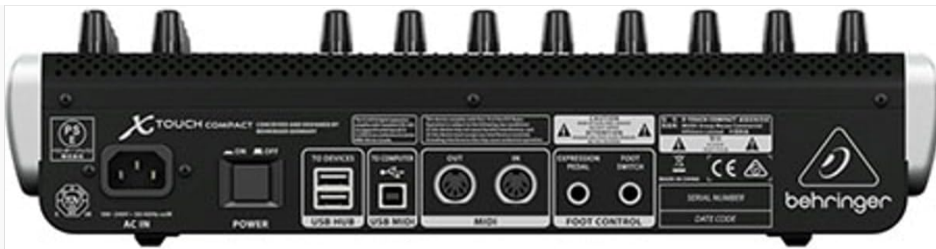
Figure 1: Rear panel connections of the X-TOUCH COMPACT, including AC IN, USB HUB, USB MIDI, MIDI IN/OUT, Expression Pedal, and Foot Switch ports.
