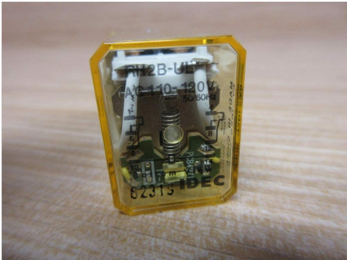
Figure 4: Close-up view of the relay's transparent casing, highlighting the model number and voltage specifications (AC110-120V, 50/60Hz).
