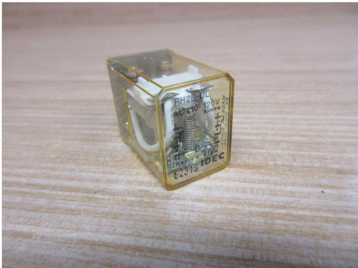
Figure 2: A single Idec RH2B-UL-AC110-120V relay, providing an angled view of the transparent casing and internal components.
