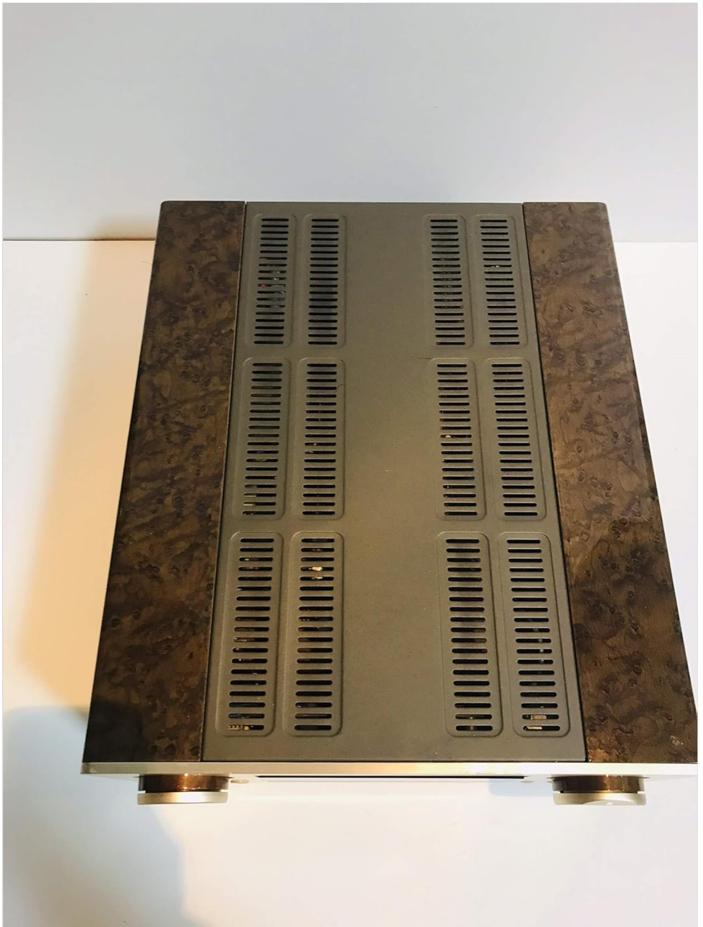
Figure 2: Top view of the Bose PLS-1310, showing the ventilation grilles.
