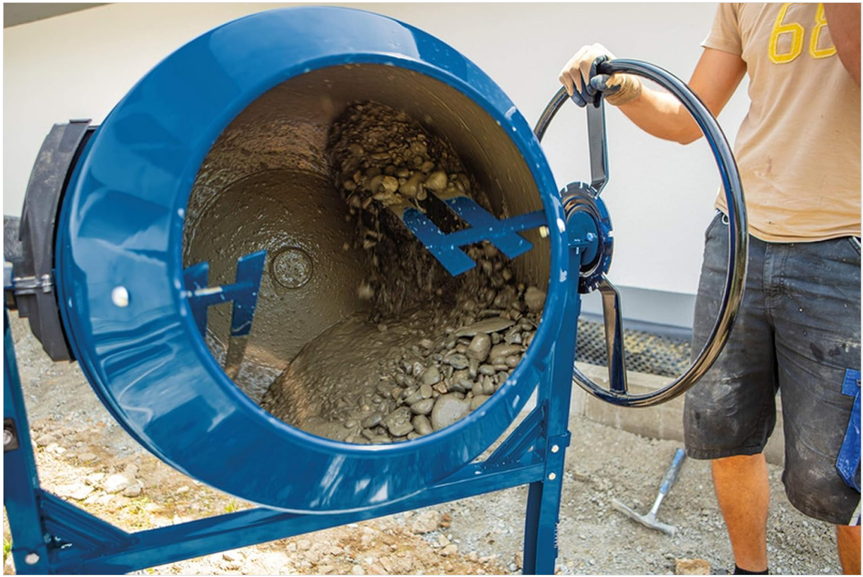
Image 4.2: A close-up view inside the blue mixer drum, showing the internal paddles actively mixing concrete with small stones and cement.
