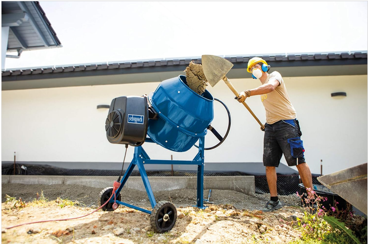
Image 4.1: An operator wearing safety gear uses a shovel to load dry materials into the rotating drum of the concrete mixer.
